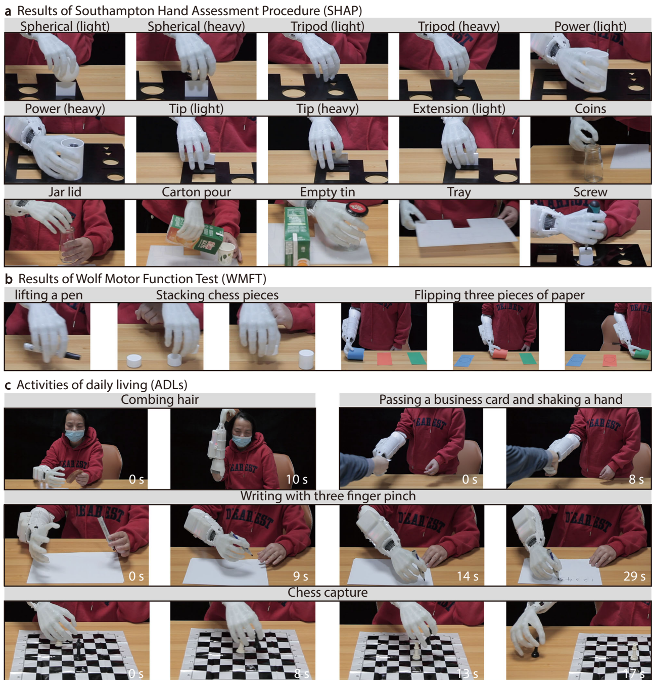
Fig. 6 | Restoring human-level hand functions via voice command. a Evaluation of the prosthetic hand's capability through Southampton Hand Assessment Procedure (SHAP), involving 15 tasks that simulate daily activities: light and heavy spherical holds, light and heavy tripod grips, light and heavy power grips, light and heavy tip pinches, light extension, manipulating coins, opening a jar lid, pouring from a carton, handling an empty tin, carrying a tray, and turning a screw. b Further
